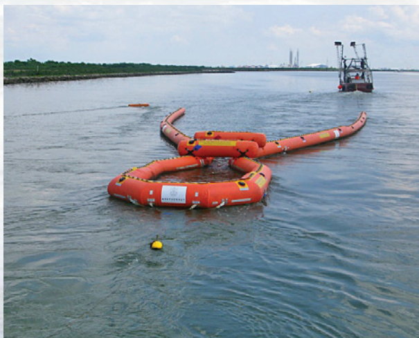
Harbour Busters proved very effective in the MACONDO response in enhancing off-shore recovery rates.
